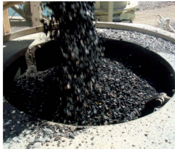
Material may be introduced into the crushing chamber via cascade, thus bypassing the rotor.
