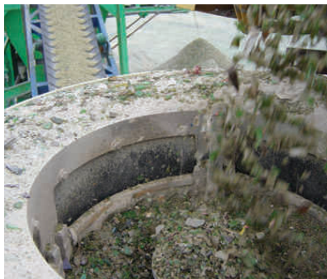
Glass can be processed and recycled using a Barmac B-Series VSI.
