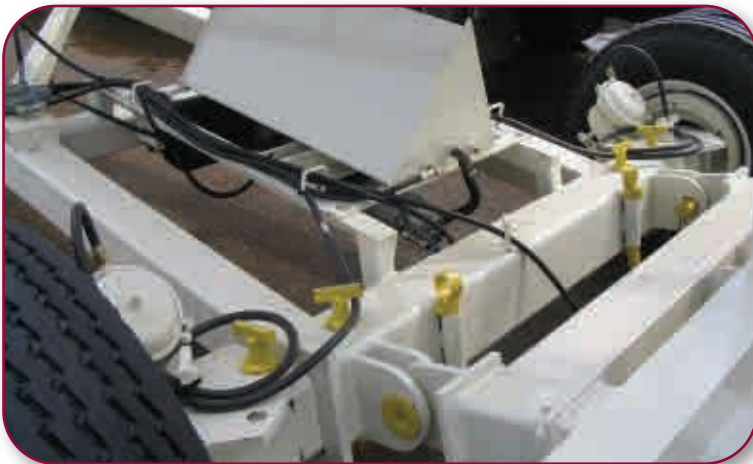
HEAVY DUTY tubular undercarriage, telescoping axle, and swivel blocks
