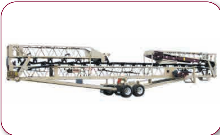
36" x 125' Portable Radial Stacking Conveyor with wrap drive, dual manual fold, power hydraulic raise, power travel and switchgear
