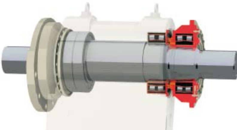
All C Series jaw crushers incorporate larger and sturdier eccentric shaft bearings than other crushers of comparable size.
